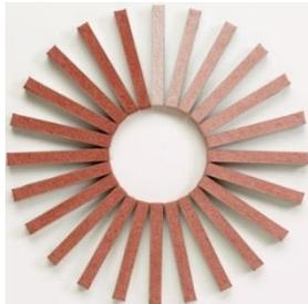
The color wheel to the left shows Synthetic Red Iron Oxide Pigment Additions from ¼% to 7% in white cement. Note how the last several samples look virtually the same. This is at or near the saturation point for this pigment.
