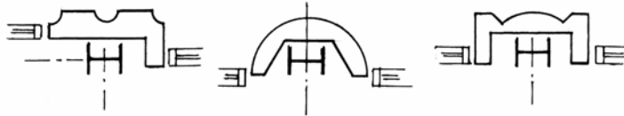
Figure B8 A concave bullnose. Figure B9 A convex bullnose. Figure B10 A partial bullnose.
